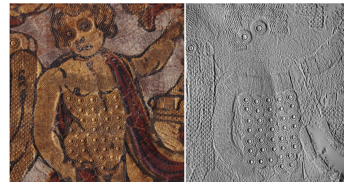
3D scan single shot accuracy: \pm 0.1 mm; point distance: 0.17 mm \sim 0.2 mm; rendering: MeshLab
