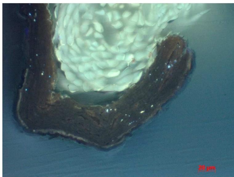
Leather metal thread cross-section, from textile CG I1bis, Civic Museum of Art of Modena, Sicily, 12<sup>th</sup> century. Image acquired with LEICA M205C stereo-microscope, Opificio delle Pietre Dure.
