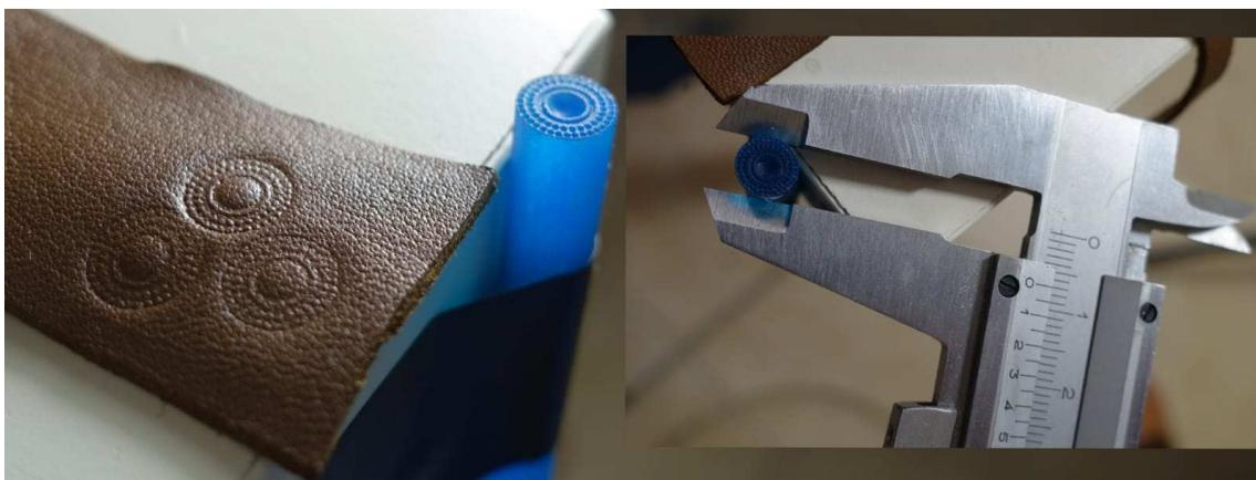
Sample of a punch mark obtained with use of 3d technologies and got from an impression on gilt leather
